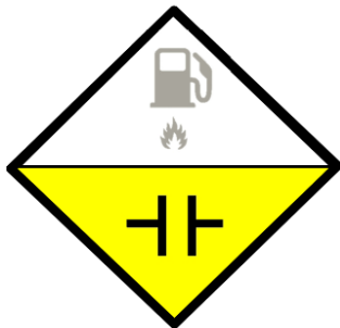
Diesel powered vehicle with super capacitor
